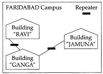
(a) Since the cabling distance between buildings GANGA and JAMUNA are quite large, so a repeater each, would ideally be needed along their path to avoid loss of signals during the course of data flow in these routes.
