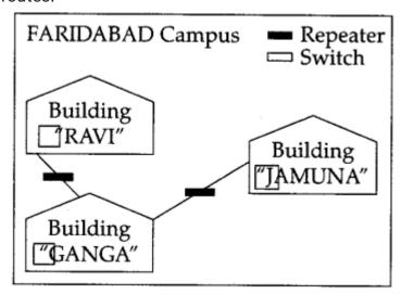
(b) In the layout a switch each would be needed in all the building, to interconnect the group of cables from the different computers in each building.
