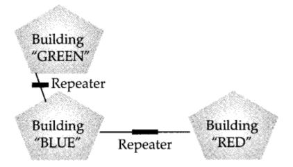
(b) In the layout a switch each, would be needed in all the buildings, to interconnect the group of cables from the different computers in each building.
