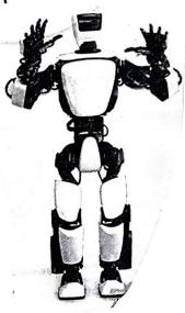
The T-HR3 is a Humanoid Robot that mimics the movements of its human operator, like a real-world avatar. It has improved controls and can walk more naturally.
